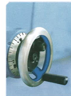
Otomatik Paso verme kolu Automatic chipping adjustment rod
