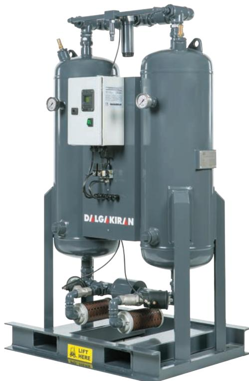
The tower being reactivated will be gradually re-pressurized at the end of its reactivation cycle before switchover take place. Purge flow and de-pressurization are in downward direction, counter flow to the drying air flow.
