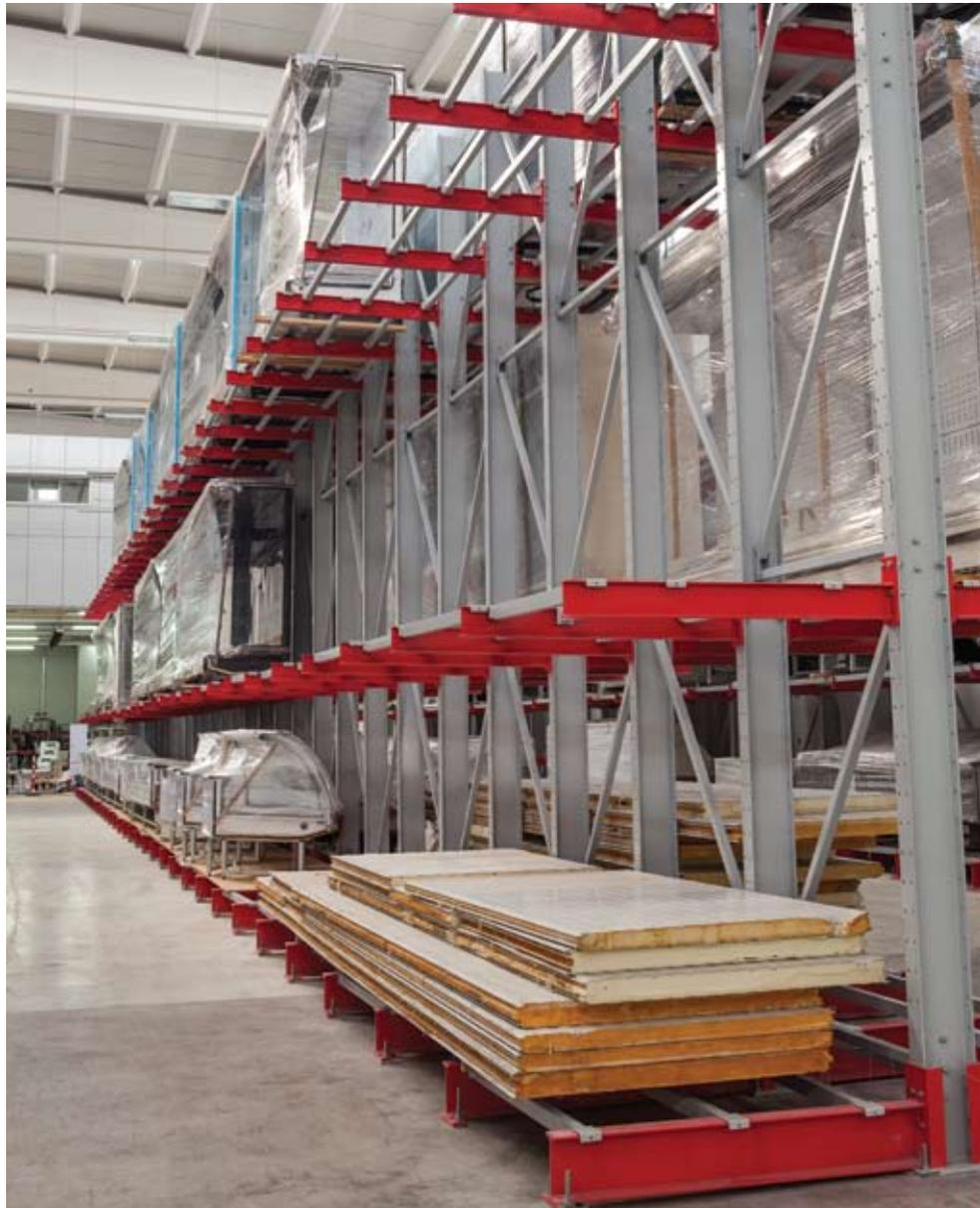
➔ Section features of the uprights and brackets to be used are variable according to the size and weight of the products to be stacked. The space between the height of the system and brackets can be adjusted in line with the stacker and the height of the warehouse.
